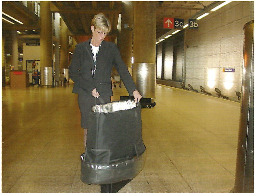
The Ground Bomb Killer is a protection device for securing suspicious items in the airport terminal
