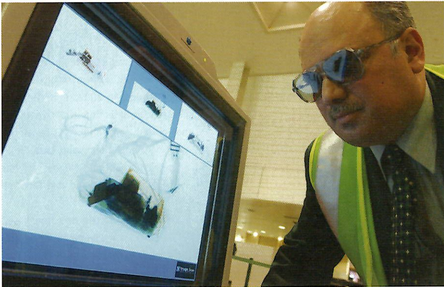
Rapiscan has introduced the Axis-3D, a three-dimensional X-ray imaging system requiring the operator to wear special glasses to view the images. The system is currently on trial at London Heathrow
